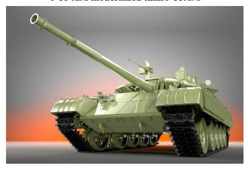
This vehicle is equipped with an automated fire control system permitting to install guided weapons, and a thermocontrol cannon casing having an anti-aircraft heavy machine gun .
