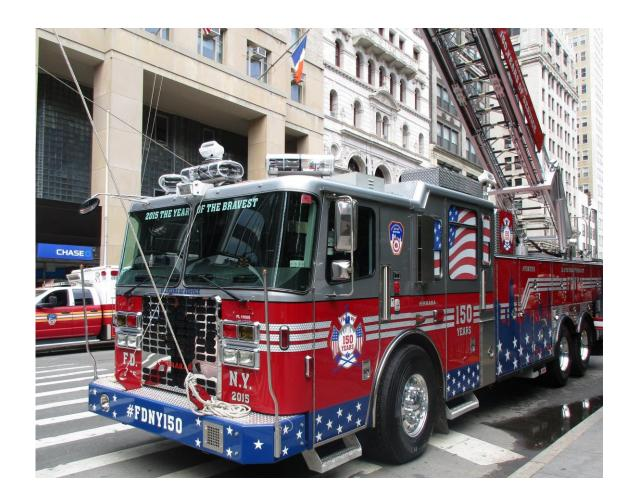
The best-known forms of the fire trucks are two types of aerial appliances: turntable ladders and hydraulic platforms. Turntable ladders have sliding ladder sections that are attached to each other and pulled upward by an extension mechanism.
