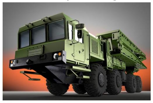
It is intended for the operational construction of bridge crossing over ditches, channels and water barriers and the passage through them of wheeled and tracked vehicles. It provides a high rate of the bridge crossing assembly, a high speed of passing equipment, high mobility during the relocation of the crossing.
