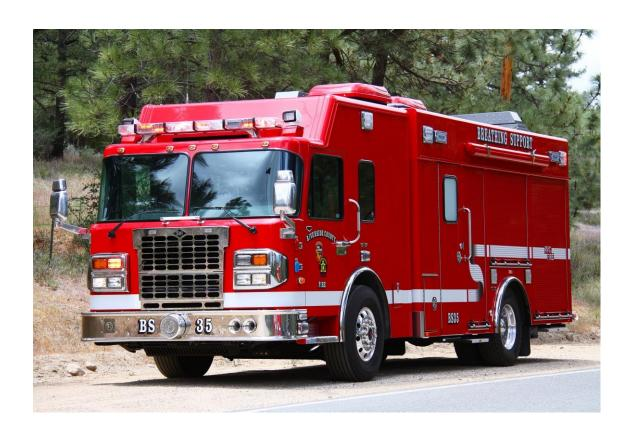
Fire engines are equipped with a large pump capable of pumping thousands of liters of water per minute. Pumpers may also carry such operational equipment as hoses, nozzles, ladders, breathing apparatus, chemical protection suits, and other firefighter gear.
