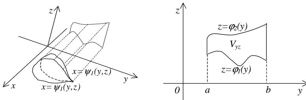
$$\iiint_V f(x, y, z) dV = \int_a^b dy \int_{\varphi_1(y)}^{\varphi_2(y)} dz \int_{\psi_1(y, z)}^{\psi_2(y, z)} f(x, y, z) dx \quad (14)$$
