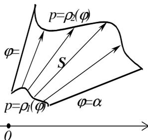
$$\iint_S \Phi(\rho; \varphi) d\rho d\varphi = \int_{\alpha}^{\beta} d\varphi \int_{\rho_1(\varphi)}^{\rho_2(\varphi)} \Phi(\rho; \varphi) d\rho \quad (4)$$
