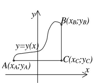
$$\int_{AB} Pdx + Qdy = \int_{AC} Pdx + Qdy + \int_{CB} Pdx + Qdy =$$
