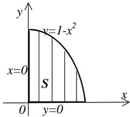
$$m = \iint_S x dx dy = \int_0^1 dx \int_0^{1-x^2} x dy = \left[ \int_0^{1-x^2} x dy = xy \Big|_0^{1-x^2} = x(1-x^2) = x - x^3 \right] =$$
