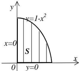
$$\iint_S \mu dx dy = \mu \int_0^1 dx \int_0^{1-x^2} dy = \left| \int_0^{1-x^2} dy = y \Big|_0^{1-x^2} = 1 - x^2 \right| = \mu \int_0^1 (1 - x^2) dx = \mu \left( x - \frac{x^3}{3} \right) \Big|_0^1 = \frac{2}{3} \mu;$$
