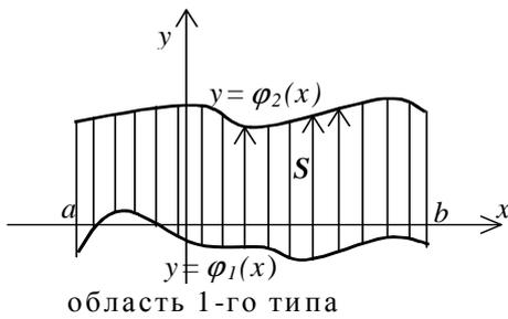
$$\iint_S f(x; y) dx dy = \int_a^b \left( \int_{\varphi_1(x)}^{\varphi_2(x)} f(x; y) dy \right) dx$$
